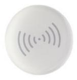
The NTAG213 on-metal tag from NXP is designed to be attached on a metal surface, utilising specially designed shielding to allow continued contactless use without interference. Operates at 13.56 MHz wireless frequency, according to the ISO 14443A standard, and contains 137 bytes of read/write space for NDEF data.
